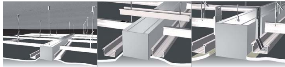
wire suspended from overhead structure - 461
