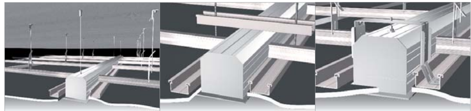
wire suspended from overhead structure - 461
