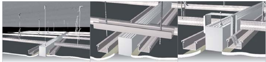
wire suspended from overhead structure - 461 direct fixed to overhead structure - 462 suspended from bracket - 463
